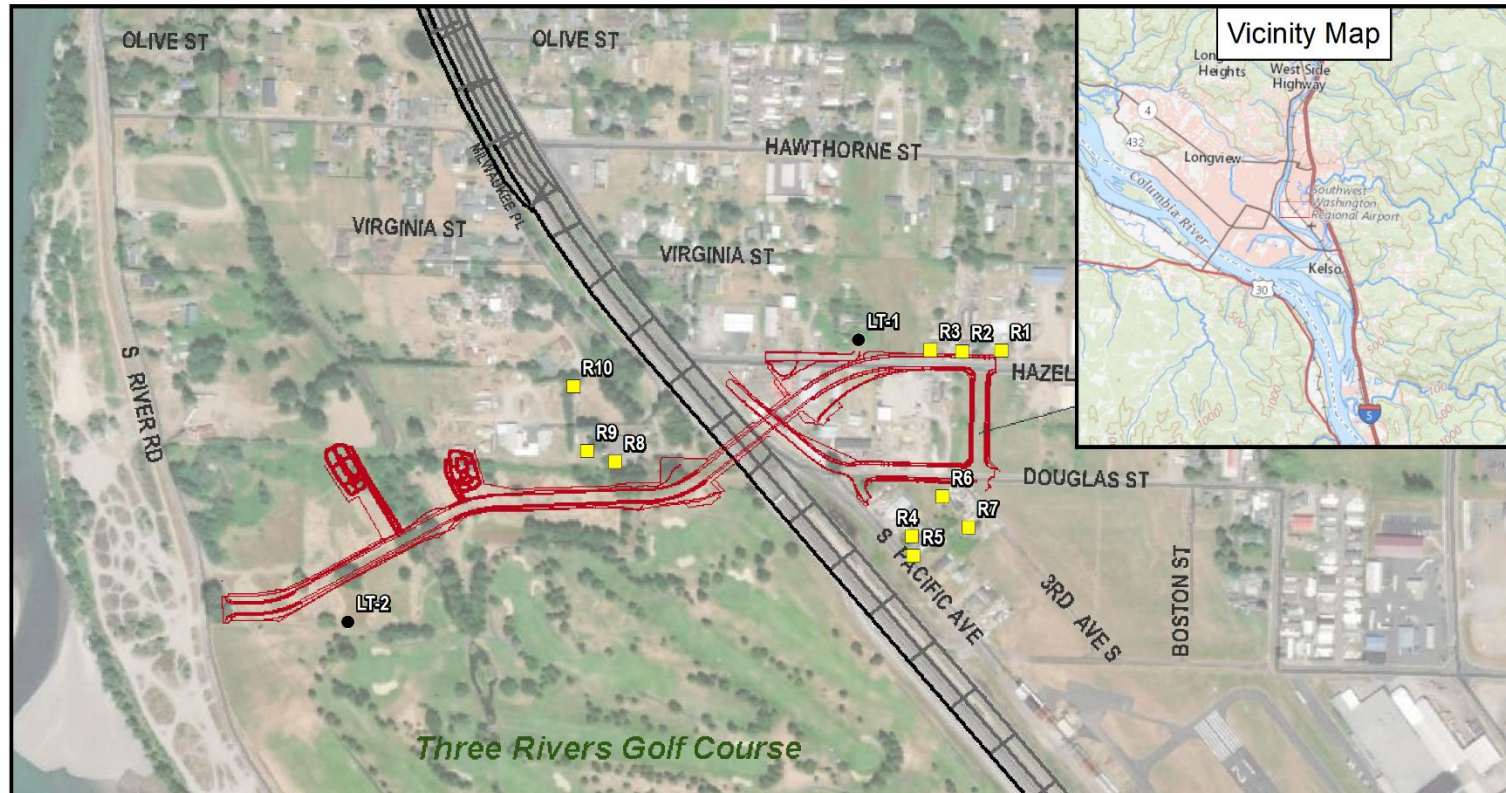
Figure 1 Vicinity Map with Noise Measurement and Noise Sensitive Receptor Locations with Build Alternative Alignment
